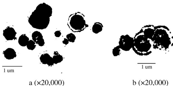
Fig. 8. Transmission electron micrograph of (a) 5-FU BSA microspheres and (b) microspheres coated by chitosan derivative.
